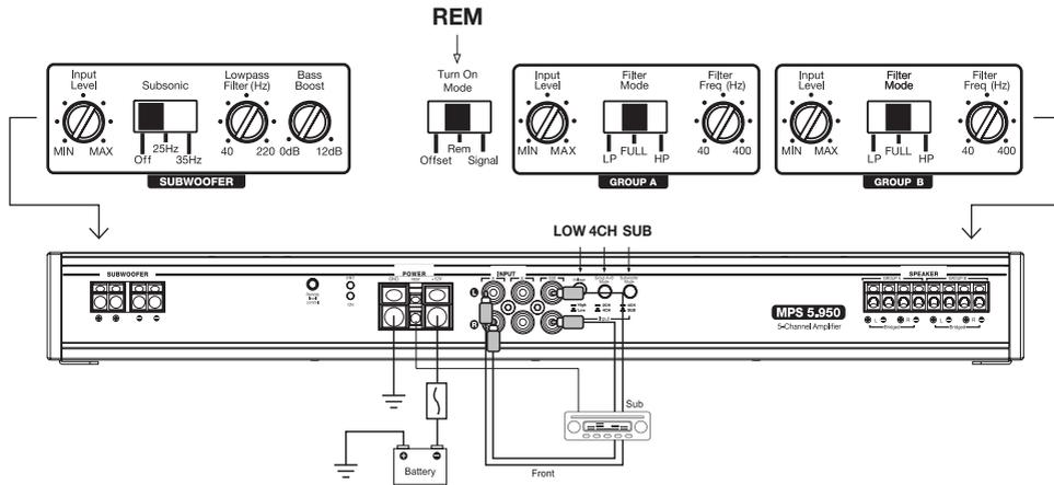
4-CHANNEL LOW LEVEL RCA INPUT ( FRONT + REAR )
