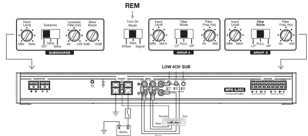
4-CHANNEL LOW LEVEL RCA INPUT ( FRONT + SUB )
